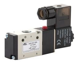
NITRA solenoid valve, 3-port (3-way), 2-position, N.C., single solenoid spring return, (1) 1/4in female NPT inlet(s), (1) 1/4in female NPT outlet(s), (1) 1/4in female NPT exhaust(s), Cv=0.89, 120 VAC, 4.5VA, 11mm DIN style wiring plug.
