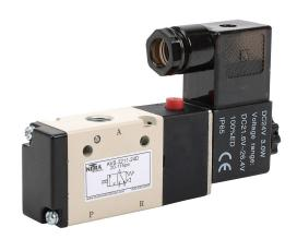
NITRA solenoid valve, 3-port (3-way), 2-position, N.C., single solenoid spring return, (1) 1/8in female NPT inlet(s), (1) 1/8in female NPT outlet(s), (1) 1/8in female NPT exhaust(s), Cv=0.78, 24 VDC, 3.0W, 11mm DIN style wiring plug.
