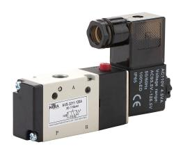
NITRA solenoid valve, 3-port (3-way), 2-position, N.C., single solenoid spring return, (1) 1/8in female NPT inlet(s), (1) 1/8in female NPT outlet(s), (1) 1/8in female NPT exhaust(s), Cv=0.78, 120 VAC, 4.5VA, 11mm DIN style wiring plug.
