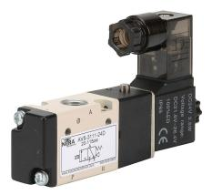
NITRA solenoid valve, 3-port (3-way), 2-position, N.C., single solenoid spring return, (1) 1/8in female NPT inlet(s), (1) 1/8in female NPT outlet(s), (1) 1/8in female NPT exhaust(s), Cv=0.67, 24 VDC, 2.5W, 9.4mm DIN style wiring plug.
