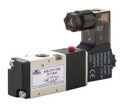
NITRA solenoid valve, 3-port (3-way), 2-position, N.C., single solenoid spring return, (1) 1/8in female NPT inlet(s), (1) 1/8in female NPT outlet(s), (1) 1/8in female NPT exhaust(s), Cv=0.67, 120 VAC, 3.5VA, 9.4mm DIN style wiring plug.
