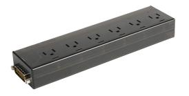
NITRA control distribution block, AC, 6 stations, 15-pin D-sub wiring connector. For use with AVS-33 and AVS-53 series valves.
