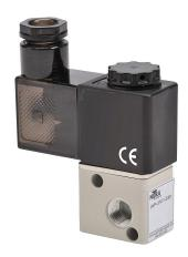
NITRA solenoid valve, 3-port (3-way), 2-position, N.C., single solenoid spring return, (2) 1/8in female NPT inlet(s), (1) 1/8in female NPT outlet(s), (1) vent hole exhaust(s), Cv=0.05, 24 VDC, 3.0W, 11mm DIN style wiring plug.
