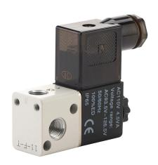
NITRA solenoid valve, 3-port (3-way), 2-position, N.C., single solenoid spring return, (2) 1/8in female NPT inlet(s), (1) 1/8in female NPT outlet(s), (1) vent hole exhaust(s), Cv=0.05, 120 VAC, 4.5VA, 11mm DIN style wiring plug.
