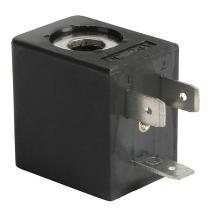
NITRA solenoid coil, 24 VDC, 3.0W. For use with AVP-31, AVS-32, AVS-33, AVS-52, AVS-53, AVS-54 series valves and ASD series soft starters.
