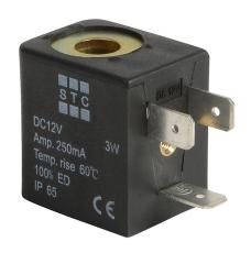
NITRA solenoid coil, 12 VDC, 3.0W. For use with AVP-31, AVS-32, AVS-33, AVS-52, AVS-53, AVS-54 series valves and ASD series soft starters.
