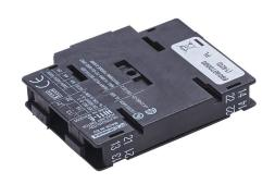
Merz auxiliary contact, left or right side mount, (1) N.O./(1) N.C. contact(s), 6A @ 120 VAC. For use with Merz ML1, ML2, ML3 door mount switch bodies -H03R(B), -H04R(B).
