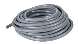
Electri-Flex Liquatite liquid-tight flexible metallic conduit, hot dipped galvanized steel, PVC jacket, 1in trade size, gray, UL-360 Listed, 100ft/30.4m coil length.
