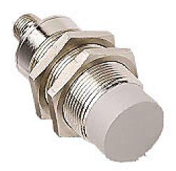
Micro Detectors inductive proximity sensor, tubular, 30mm diameter x 60mm body, nickel-plated brass housing, PNP, N.O. output, 20mm sensing distance, non-flush, 150 Hz switching frequency, IP67, 4-pin M12 quick-disconnect.
