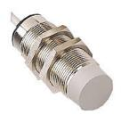
Micro Detectors inductive proximity sensor, tubular, 30mm diameter x 60mm body, nickel-plated brass housing, PNP, N.O. output, 15mm sensing distance, non-flush, 300 Hz switching frequency, IP67, pigtail.
