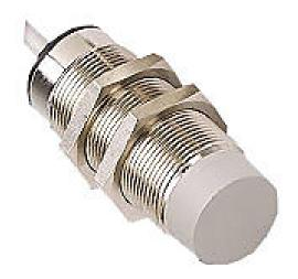
Micro Detectors inductive proximity sensor, tubular, 30mm diameter x 60mm body, nickel-plated brass housing, NPN, N.O. output, 20mm sensing distance, non-flush, 150 Hz switching frequency, IP67, pigtail.
