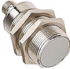
Micro Detectors inductive proximity sensor, tubular, 30mm diameter x 60mm body, nickel-plated brass housing, NPN, N.O. output, 15mm sensing distance, flush, 150 Hz switching frequency, IP67, 4-pin M12 quick-disconnect.
