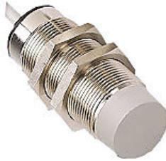
Micro Detectors inductive proximity sensor, tubular, 30mm diameter x 60mm body, nickel-plated brass housing, NPN, N.O. output, 15mm sensing distance, non-flush, 300 Hz switching frequency, IP67, pigtail.
