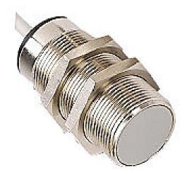
Micro Detectors inductive proximity sensor, tubular, 30mm diameter x 60mm body, nickel-plated brass housing, NPN, N.O. output, 10mm sensing distance, flush, 300 Hz switching frequency, IP67, pigtail.
