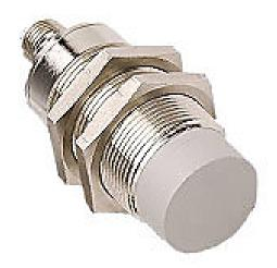
Micro Detectors inductive proximity sensor, tubular, 30mm diameter x 60mm body, nickel-plated brass housing, NPN/PNP, N.O. output, 15mm sensing distance, non-flush, 150 Hz switching frequency, IP67, 4-pin M12 quick-disconnect.
