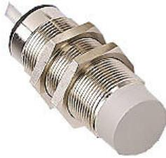
Micro Detectors inductive proximity sensor, tubular, 30mm diameter x 60mm body, nickel-plated brass housing, NPN/PNP, N.O. output, 15mm sensing distance, non-flush, 150 Hz switching frequency, IP67, pigtail.
