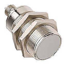
Micro Detectors inductive proximity sensor, tubular, 30mm diameter x 60mm body, nickel-plated brass housing, NPN/PNP, N.O. output, 10mm sensing distance, flush, 150 Hz switching frequency, IP67, 4-pin M12 quick-disconnect.
