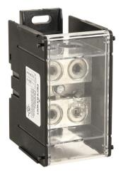
Penn-Union open splicer/reducer block, finger-safe, 760A, 1-pole, line side: 2 openings accept 500 MCM to 4 AWG Cu/AL, load side: 2 openings accept 500 MCM to 4 AWG Cu/AL, DIN rail or panel mount, UL 1953 listed.
