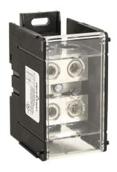
Penn-Union open splicer/reducer block, finger-safe, 620A, 1-pole, line side: 2 openings accept 350 MCM to 6 AWG Cu/AL, load side: 2 openings accept 350 MCM to 6 AWG Cu/AL, DIN rail or panel mount, UL 1953 listed.
