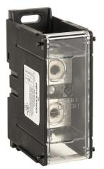
Penn-Union open splicer/reducer block, finger-safe, 380A, 1-pole, line side: 1 openings accept 500 MCM to 4 AWG Cu/AL, load side: 1 openings accept 500 MCM to 4 AWG Cu/AL, DIN rail or panel mount, UL 1953 listed.
