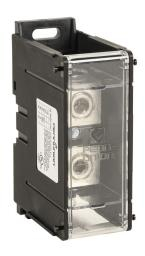
Penn-Union open splicer/reducer block, finger-safe, 310A, 1-pole, line side: 1 openings accept 350 MCM to 6 AWG Cu/AL, load side: 1 openings accept 350 MCM to 6 AWG Cu/AL, DIN rail or panel mount, UL 1953 listed.
