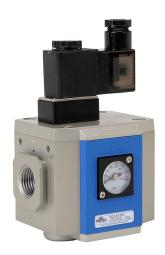
NITRA soft start valve, 3-port (3-way), 2-position, single solenoid spring return, N.C., 1/2in female NPT inlet(s), 1/2in female NPT outlet(s), 1/2in female NPT exhaust(s), Cv=24, 24 VDC operating voltage. For use with Ax-44 series air prep components.
