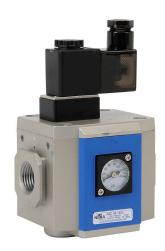
NITRA soft start valve, 3-port (3-way), 2-position, single solenoid spring return, N.C., 1/2in female NPT inlet(s), 1/2in female NPT outlet(s), 1/2in female NPT exhaust(s), Cv=24, 120 VAC operating voltage. For use with Ax-44 series air prep components.
