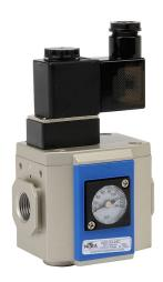
NITRA soft start valve, 3-port (3-way), 2-position, single solenoid spring return, N.C., 3/8in female NPT inlet(s), 3/8in female NPT outlet(s), 3/8in female NPT exhaust(s), Cv=15, 24 VDC operating voltage. For use with Ax-33 series air prep components.
