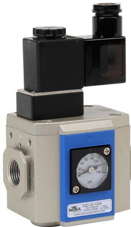
NITRA soft start valve, 3-port (3-way), 2-position, single solenoid spring return, N.C., 3/8in female NPT inlet(s), 3/8in female NPT outlet(s), 3/8in female NPT exhaust(s), Cv=15, 120 VAC operating voltage. For use with Ax-33 series air prep components.
