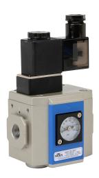
NITRA soft start valve, 3-port (3-way), 2-position, single solenoid spring return, N.C., 1/4in female NPT inlet(s), 1/4in female NPT outlet(s), 3/8in female NPT exhaust(s), Cv=12, 24 VDC operating voltage. For use with Ax-32 series air prep components.
