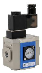
NITRA soft start valve, 3-port (3-way), 2-position, single solenoid spring return, N.C., 1/4in female NPT inlet(s), 1/4in female NPT outlet(s), 3/8in female NPT exhaust(s), Cv=12, 120 VAC operating voltage. For use with Ax-32 series air prep components.
