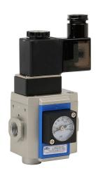
NITRA soft start valve, 3-port (3-way), 2-position, single solenoid spring return, N.C., 1/4in female NPT inlet(s), 1/4in female NPT outlet(s), 1/4in female NPT exhaust(s), Cv=7.5, 24 VDC operating voltage. For use with Ax-22 series air prep components.
