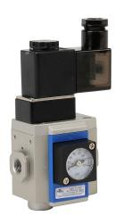
NITRA soft start valve, 3-port (3-way), 2-position, single solenoid spring return, N.C., 1/8in female NPT inlet(s), 1/8in female NPT outlet(s), 1/4in female NPT exhaust(s), Cv=7, 24 VDC operating voltage. For use with Ax-21 series air prep components.
