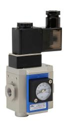
NITRA soft start valve, 3-port (3-way), 2-position, single solenoid spring return, N.C., 1/8in female NPT inlet(s), 1/8in female NPT outlet(s), 1/4in female NPT exhaust(s), Cv=7, 120 VAC operating voltage. For use with Ax-21 series air prep components.
