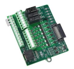
Toshiba AS3 series relay/analog combo module, Analog Input: 3-channel, current/voltage, Analog Output: 2-channel, current/voltage, Discrete Input: 6-point, Discrete Output: 3-point, relay, (1) Form C (SPDT) relay, (2) Form A (SPST) relays.
