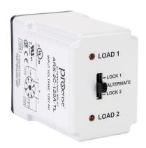
ProSense alternating relay, socket mount, finger-safe, 120 VAC coil voltage, DPDT, (2) N.O., (2) N.C., 10A contact rating, 8-pin, LED indicator(s). Relay becomes UL listed when used with 70169-D relay socket.
