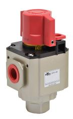
NITRA shut-off valve, 3-port (3-way), 2-position, twist, N.C., 1/2in female NPT inlet(s), 1/2in female NPT outlet(s), 1/2in female NPT exhaust(s). For use with Ax-44 series air prep components.
