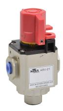
NITRA shut-off valve, 3-port (3-way), 2-position, twist, N.C., 1/8in female NPT inlet(s), 1/8in female NPT outlet(s), 1/4in female NPT exhaust(s). For use with Ax-21 series air prep components.
