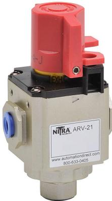
NITRA shut-off valve, 3-port (3-way), 2-position, twist, N.C., 1/8in female NPT inlet(s), 1/8in female NPT outlet(s), 1/4in female NPT exhaust(s). For use with Ax-21 series air prep components.
