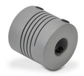
AutomationDirect encoder coupling, 3/8in bore, aluminum alloy body, setscrew. For use with Koyo TRDA-20 and TRDA-25 series encoders.
