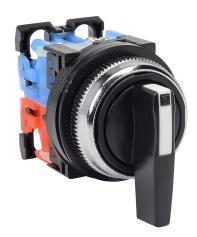
Fuji Electric selector switch, 30mm, 3-position, spring return from right to center / manual return from left to center, (1) N.O./(1) N.C. contact(s), plastic base, metal bezel, Operator: black, lever, 35mm, round, plastic.
