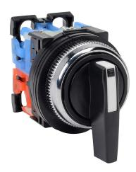
Fuji Electric selector switch, 30mm, 3-position, maintained, (1) N.O./(1) N.C. contact(s), plastic base, metal bezel, Operator: black, lever, 35mm, round, plastic.
