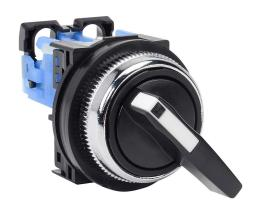
Fuji Electric selector switch, 30mm, 2-position, maintained, (1) N.O. contact(s), plastic base, metal bezel, Operator: black, lever, 35mm, round, plastic.
