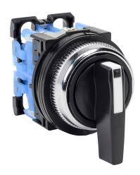
Fuji Electric selector switch, 30mm, 3-position, spring return from left and right to center, (2) N.O. contact(s), plastic base, metal bezel, Operator: black, lever, 35mm, round, plastic.
