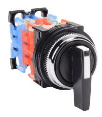
Fuji Electric selector switch, 30mm, 5-position, maintained, (2) N.O./(2) N.C. contact(s), plastic base, metal bezel, Operator: black, lever, 35mm, round, plastic.
