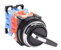
Fuji Electric selector switch, 30mm, 4-position, maintained, (2) N.O./(2) N.C. contact(s), plastic base, metal bezel, Operator: black, lever, 35mm, round, plastic.
