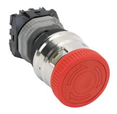
Fuji Electric emergency stop pushbutton, IP65, 30mm, push to lock, turn to reset, (1) N.O./(2) N.C. contact(s), plastic base, metal bezel, silver, Operator: red, mushroom, 44mm, mushroom, plastic.
