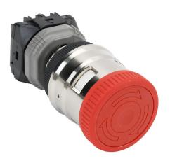
Fuji Electric emergency stop pushbutton, IP65, 30mm, push to lock, turn to reset, (1) N.C. contact(s), plastic base, metal bezel, silver, Operator: red, mushroom, 44mm, mushroom, plastic.
