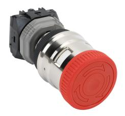
Fuji Electric emergency stop pushbutton, IP65, 30mm, push to lock, turn to reset, (1) N.C. contact(s), plastic base, metal bezel, silver, Operator: red, mushroom, 44mm, mushroom, plastic.
