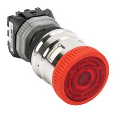
Fuji Electric emergency stop pushbutton, IP65, 30mm, push to lock, turn to reset, interlocked LED illuminated, (1) N.O./(2) N.C. contact(s), plastic base, metal bezel, silver, Operator: red, mushroom, 44mm, mushroom, plastic, 24 VAC/VDC, full voltage.
