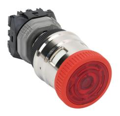
Fuji Electric emergency stop pushbutton, IP65, 30mm, push to lock, turn to reset, interlocked LED illuminated, (1) N.C. contact(s), plastic base, metal bezel, silver, Operator: red, mushroom, 44mm, mushroom, plastic, 24 VAC/VDC, full voltage.
