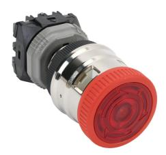
Fuji Electric emergency stop pushbutton, IP65, 30mm, push to lock, turn to reset, LED illuminated, (1) N.C. contact(s), plastic base, metal bezel, silver, Operator: red, mushroom, 44mm, mushroom, plastic, 24 VAC/VDC, full voltage.
