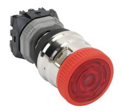
Fuji Electric emergency stop pushbutton, IP65, 30mm, push to lock, turn to reset, LED illuminated, (1) N.C. contact(s), plastic base, metal bezel, silver, Operator: red, mushroom, 44mm, mushroom, plastic, 24 VAC/VDC, full voltage.
